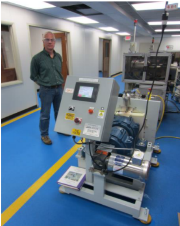
Figure 2.4 - Photo of Main Shaft Seal Test Arrangement
